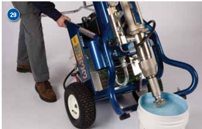
Insert siphon end of pump into pail.
