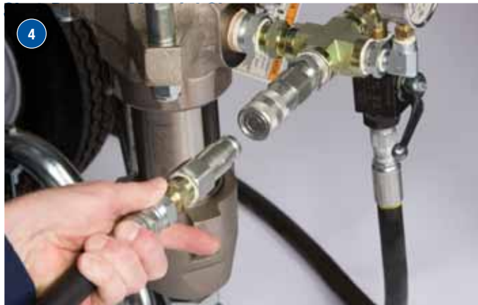
Connect jump hose to Graco pump.
