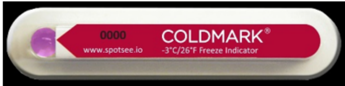
Freeze Indicator, Un-Broken (Clear), Broken (Violet)
