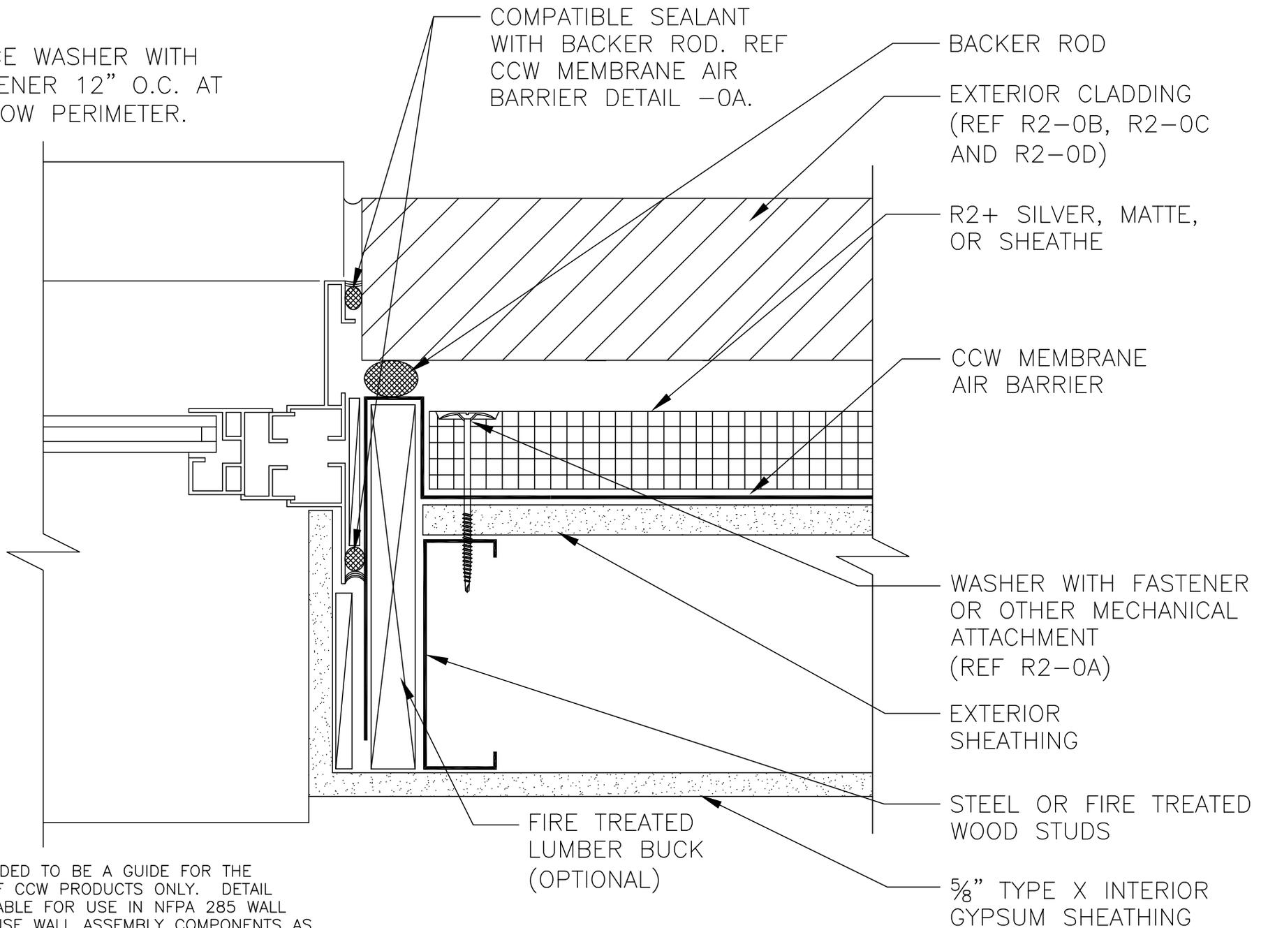
DETAIL IS INTENDED TO BE A GUIDE FOR THE INSTALLATION OF CCW PRODUCTS ONLY. DETAIL SHOWN IS SUITABLE FOR USE IN NFPA 285 WALL ASSEMBLIES. USE WALL ASSEMBLY COMPONENTS AS LISTED IN R2-0B, R2-0C AND R2-0D DETAILS.
